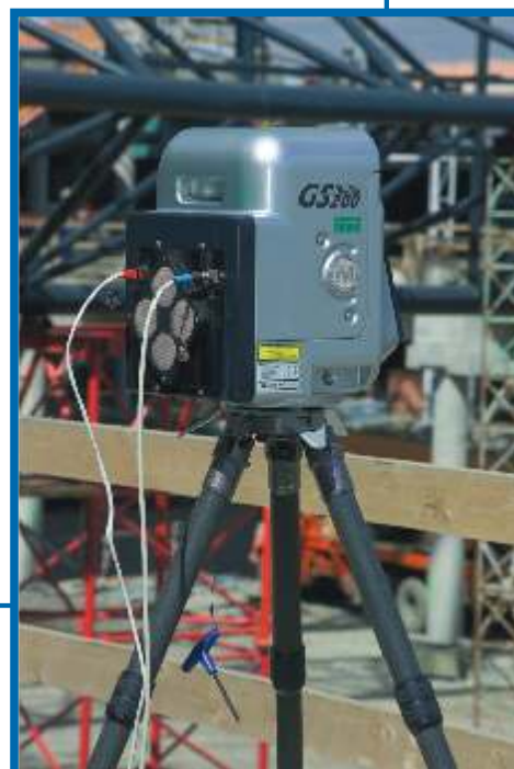
Detailed assembly precision check on a roof structure
