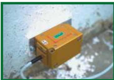
Vibration sensor on the wall
